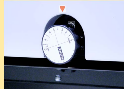
Adjustment of strap tension by handwheel
